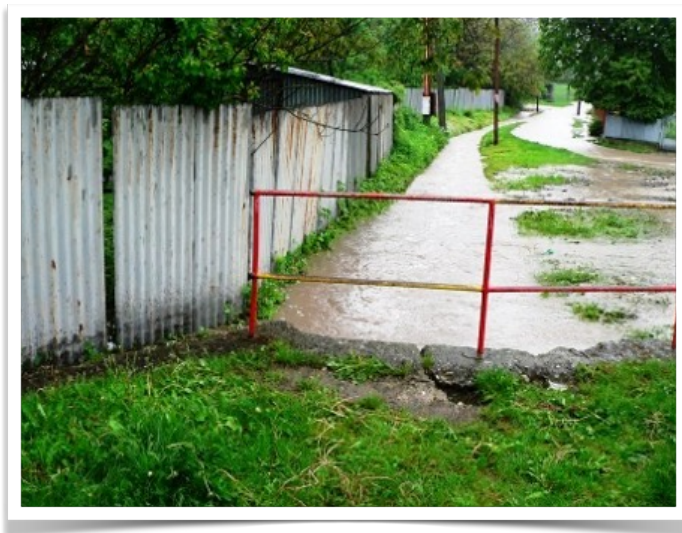
Left: An impermeable asphalted pavement and road allow the rainwaters to rush down faster, forming a flooded trail, stopped by a berm temporarily.
